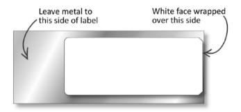
Smallest recommended bending diameter of the Confidex ESD On Metal Label™ is 100mm. For optimal performance please bend the label in the orientation shown below.
